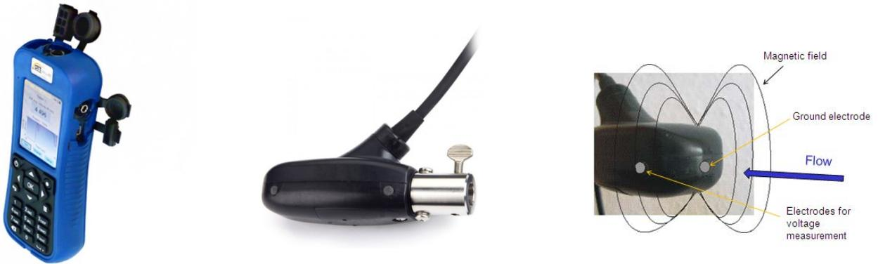
The service life of the OTT MF-Pro should be about ten years. It is an all-electronic device with no moving parts. The sensor is separate from the handset and is also calibrated separately from the handset. This means if the sensor or handset fail, the user could just order the needed component without having to replace the entire setup. This is a relatively new instrument so repair costs are really just estimates at this point.
